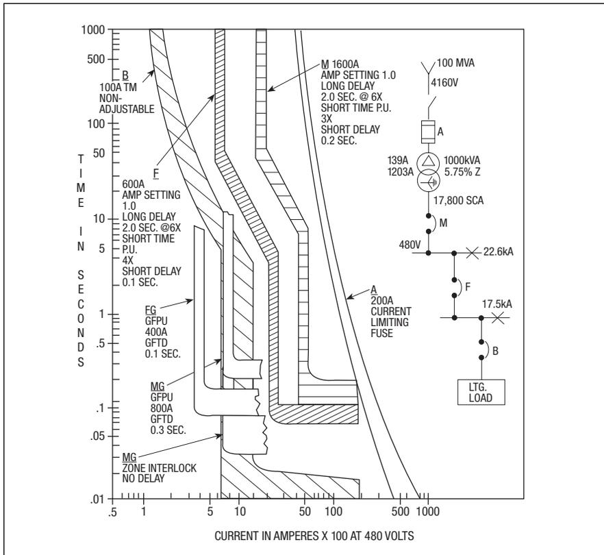
Figure 3 — Typical System — Selectively Coordinated (NEMA AB3)
