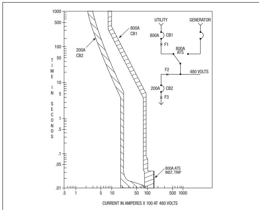
Figure 5 — System Response to Downstream Overcurrent at F3
